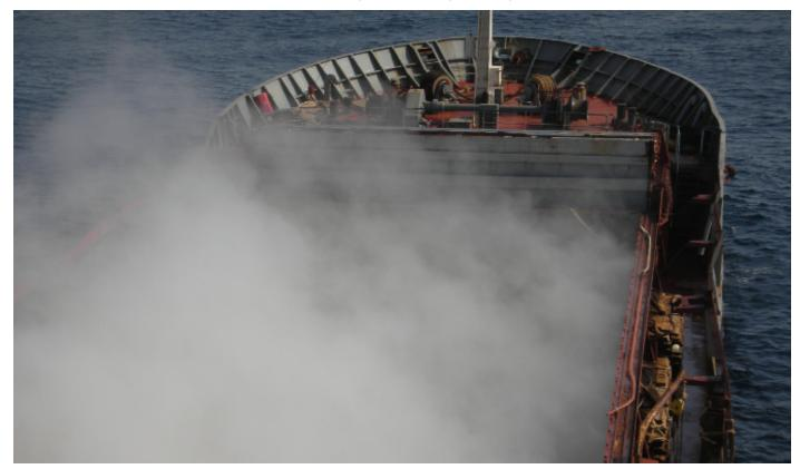
Vessel suffering from DRI self-heating
