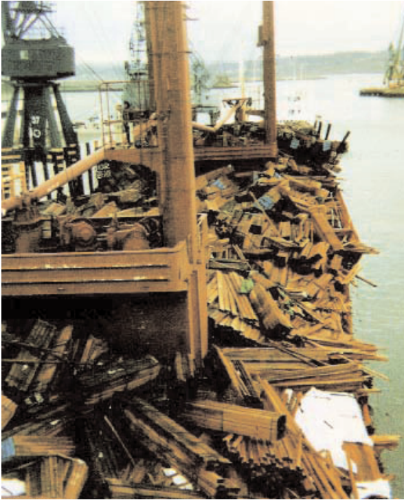
Similar cargo, poorly stowed, improperly secured, widespread gaps in cargo. Total collapse of stowage, 50% deck cargo bundles lost overboard, widespread structural damage to vessel
