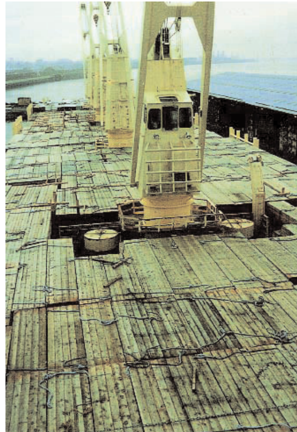
An example of a full timber deck cargo, compactly stowed, ends butted prior to securing with chain lashings 1.5m apart
