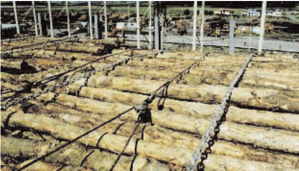
The correct use of wiggle-wires through snatch blocks – used to bind and consolidate the log stow – independent of the number and pitch of cross-lashings required. Photo shows chain cross-lashings pitched 3m apart for stow not exceeding 4m in height above the weatherdeck at the ship's side
