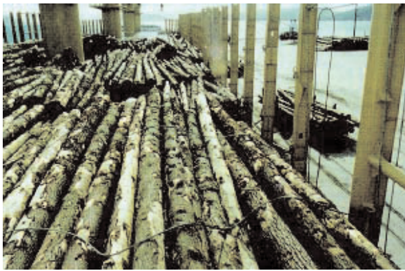
Rigging hog wires for deck-stowed log cargo, as required by the IMO Code of Safe Practice for Ships Carrying Timber Deck Cargoes, 1991
