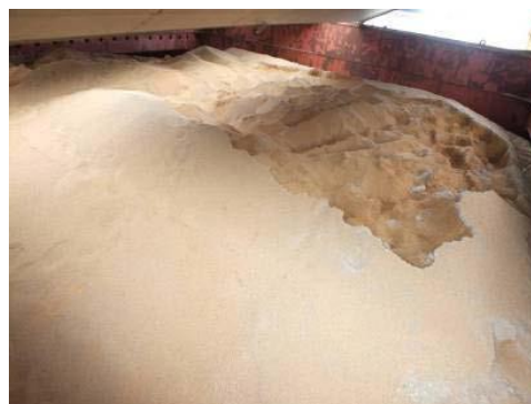
Grain cargo - wet damage from leaking hatch cover
