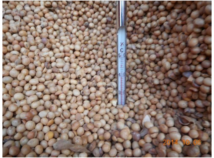
Checking and recording cargo temperature
