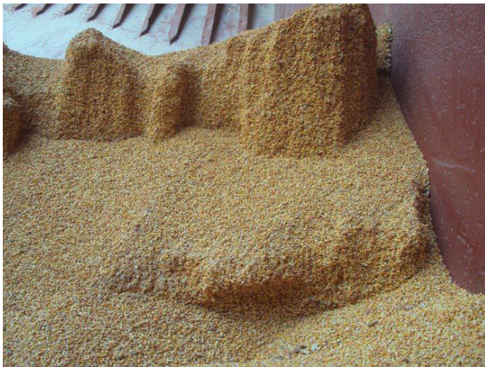
Heat damaged grain – stowed next to engine room bulkhead
