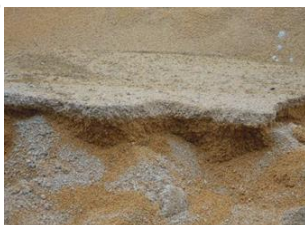
Caking from self-heating
