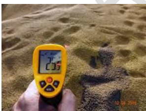
Cargo temperature on loading should not change much during voyage. An increase in cargo temperature is an indication of self-heating.
