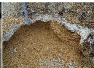
Visible mould from self heating
