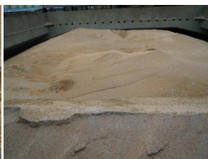
Discolouration from self-heating
