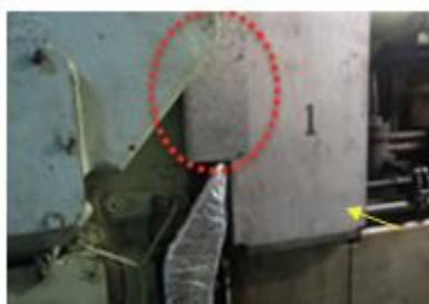
Shielding to protect the turbocharger
